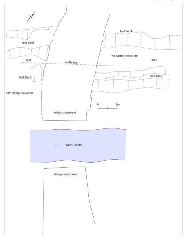
**Figure 8:** Plan drawing of the bridge abutments, and the leat in the vicinity of the northern bridge abutment where excavations were carried out.
