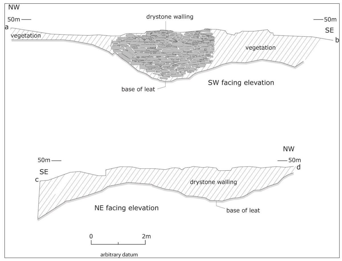
Figure 9: The southwest- and northeast-facing elevations of the northern bridge abutment
