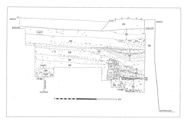
Section drawing of the 1994 excavation showing the deeply stratified deposits behind the upstanding town wall.
